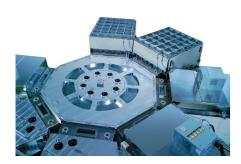
CMD series are single-substrate CVD system for deposition of a-Si film, silicon oxide film and nitride film using SiH4 or TEOS.
